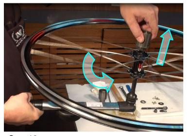
Step 12 Screw out cassette body by turning wheel.
