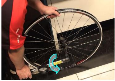
Step 11 Support the wheel on a stable surface & loosen the fixed bolt which secures the cassette body to the hub shell.
