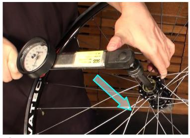
Step 10 Insert 12mm allen key into "Fixed Bolt" located inside hub shell.
