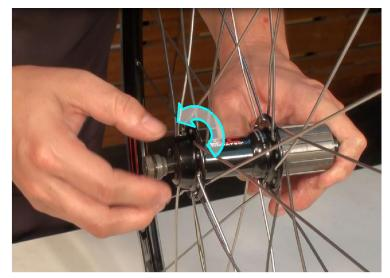
Step 4 Screw out & remove cone.
