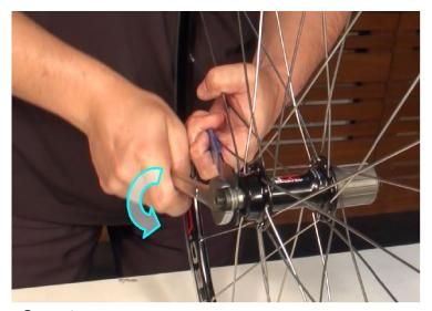
Step 1 Loosen "Cone" & nut by wrench key 15mm & 17mm.
