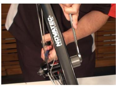
Step 2 Loosen "Cone" & axle by wrench key 15mm & 17mm.
