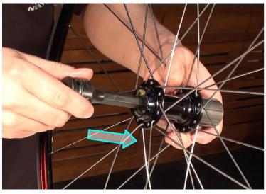
Step 2 Insert allen key 12mm & screw it by hand in order to connect "Fixed Bolt" with cassette body.
