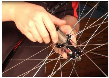
Step 22 Check smoothness of rotation and check if cassette body works properly.
