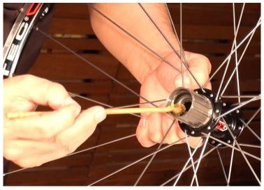
Step 8 Grease cups on both sides of hub.
