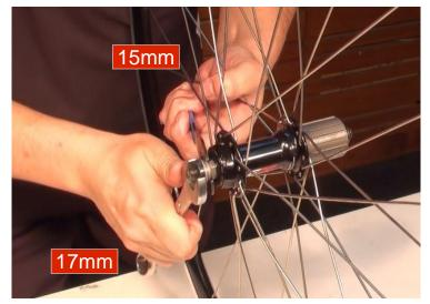
Step 18 Hold "Cone" and tighten "Nut" in clockwise direction.
