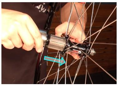
Step 21 Press "Oil Seal" to correct position.
