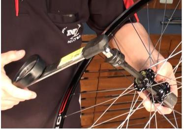
Step 3 Insert torque wrench to allen key 12mm.
