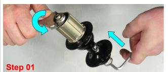
Insert allen key to axle and hold it. Unscrew right side cap by wrench key by anti-clockwise direction.
