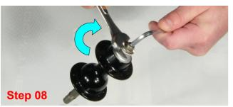
Hold allen key & by wrench key tight Campy left side cap by clockwise direction.
