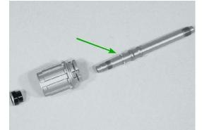
Step 06 Take a part axle & cassbody. Remember position of Washer 197 !!! This position of Washer 197 is only for Shim. !!!
