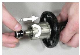
**Step 11** Insert side cap into axle & screw it in by clockwise direction.
