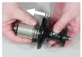
**Step 03** Remove axle with cass.body from hub shell.
