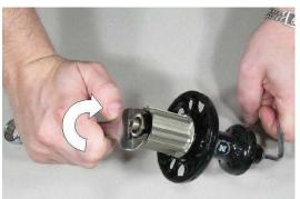
**Step 12** Insert allen key into axle & hold it. Tight side cap by wrench key by clockwise direction.
