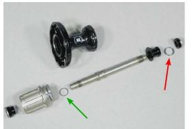
Step 07 Position of Washer 199 & Washer 197. This position is using only for Shim. type !!!
