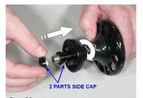
Step 09 Insert two parts of side cap into axle & screw it in by hand. There is no washer between two parts of side cap in Campy type !!!
