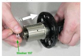
Step 11 Insert into axle cass.body & then insert Washer 197. This position of Washer 197 is only for Campy !!!
