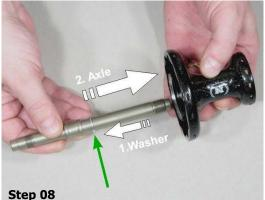
Insert Washer 197 into the axle & place the axle into the hub shell. Be sure with correct position of Washer 197.
