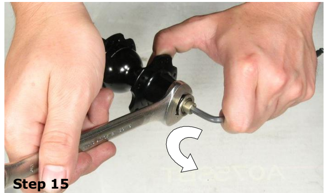
Step 14 Then tighten the hub by using wrench key in clockwise direction.
