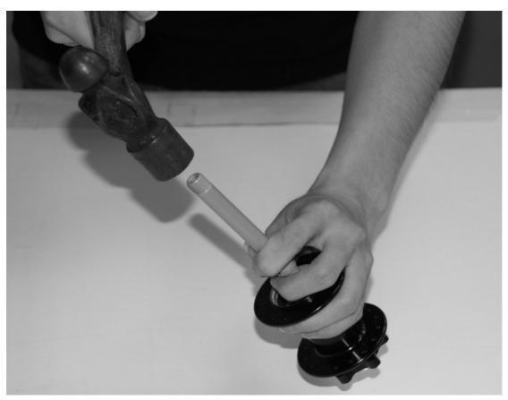
5. Put axle [or any tube] inside to the hub to tap up and change position around inside to push the farther sealed bearing out.
