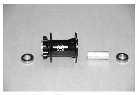
8. After disassemble the parts of hub.
