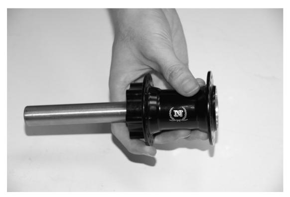
5. Fasten the Expander Tube into hub.
