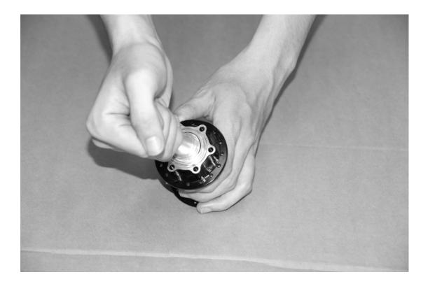
3. Use any tube to take out end cup with rubber O-ring.
