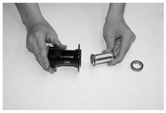
9. Take out the inner tube and sealed bearing
