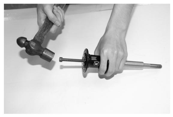
8. Use hammer to tap up the tool with sealed bearing.
