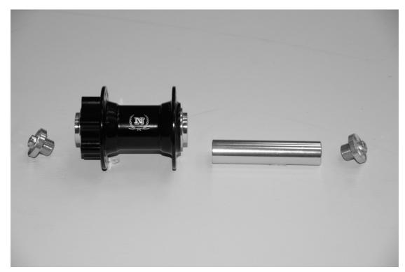
1. Un-tighten side cap and remove tube
