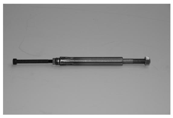
"Tools 661" for bearing disassembly.
